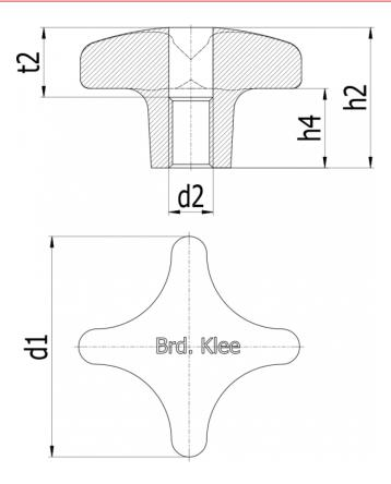
$\begin{array}{lll} d1 & = 50 \\ d2 & = M10 \\ h2 & = 32 \\ h4 & = 18 \\ t2 & = 16 \\ Weight in (g) = 108 \end{array}$
